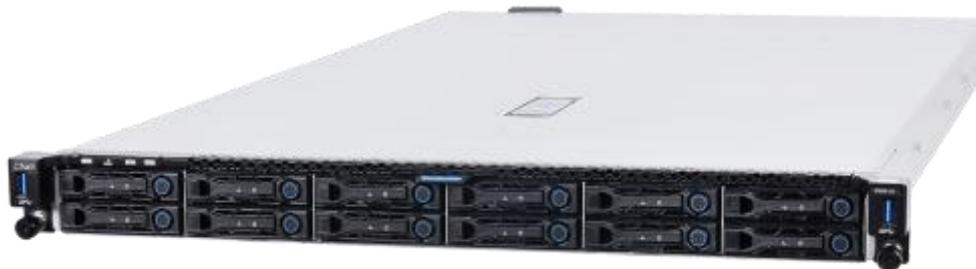
*Figure 2 High density fast storage NVMe server*
